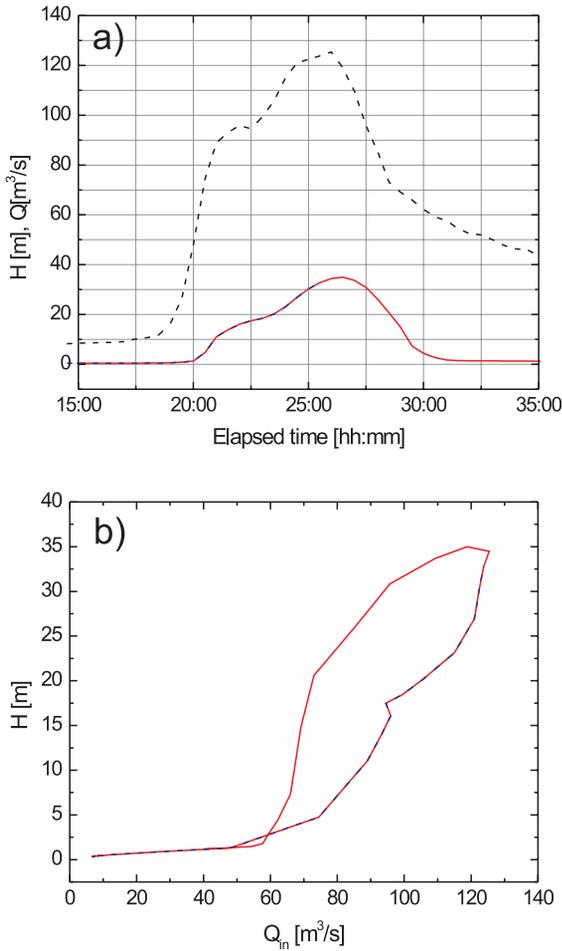
Fig. 10: Model results of the event (Fig. 5c) passing through the system on Fig. 8. a) Dashed line presents the input flow rates, full lines give the level hydrogram  $h_2$  b) Flow-Level curve.
