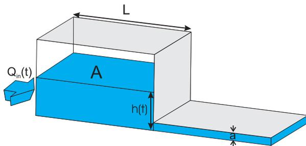
Fig. 11: Simple model of a large channel ending with restriction. The length of the entrance channel is  $L$ ,  $a$  is the height of the restriction,  $A$  the surface area of the water prior to it and  $Q_{in}(t)$  the input flow hydrograph.
