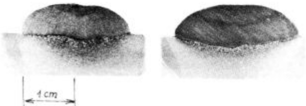
Slika 4: Videz preseka navara s trojno elektrodo ( \phi 1,6 mm) pod legiranim praškom: a) "U-Mo-6" in b) "BM-2" ( I = 185 A/žico, U = 44 V) Figure 4: Macrography of the cross-section of the submerged arc surfacing made with triple electrode ( \phi_{\text{wire}} = 1.6 mm) and with alloyed fluxes: a) "U-Mo-6" and b) "BM-2" ( I = 185 A/wire, U = 44 V)
