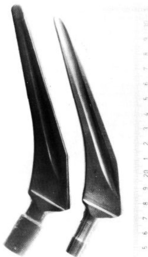
Slika 1: Neobdelan in delno obdelan izkovek Figure 1: Wrought and rough-machined forging
