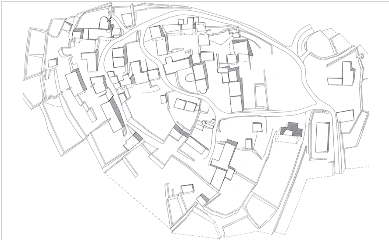
Figure 2: The axonometry of terraces and terraced excavations for houses' foundations in the village of Glem shows that all old settlements in northern Istria were built in a terraced manner (Pikel, 1993, 112)
