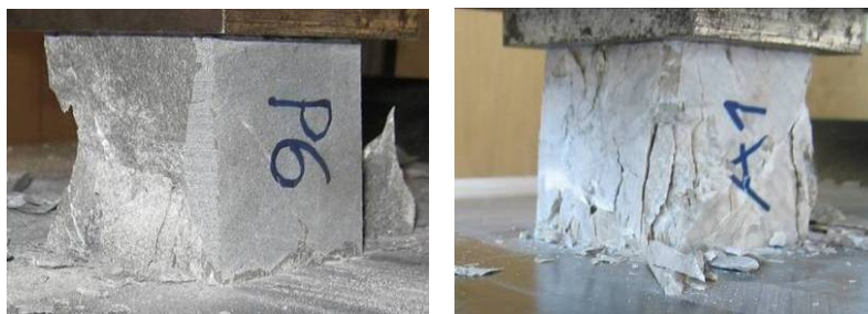
Slika 5.6: Preiskave tlačne trdnosti peščenjaka in apnenca Fig. 5.6: Compressive strength tests on sandstone and limestone specimens
