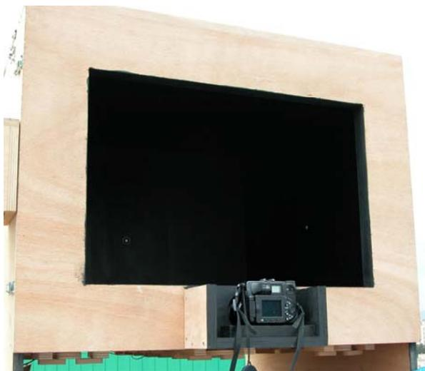
Fig. 5.3. Position of the digital camera with fish-eye lens (black surface is the opening (60 cm x 40 cm) into the scale model)
