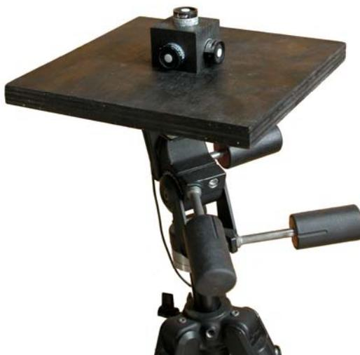
*Fig. 1.11. Illuminance sensors with wooden cube fixed on a plate and on a tripod*
