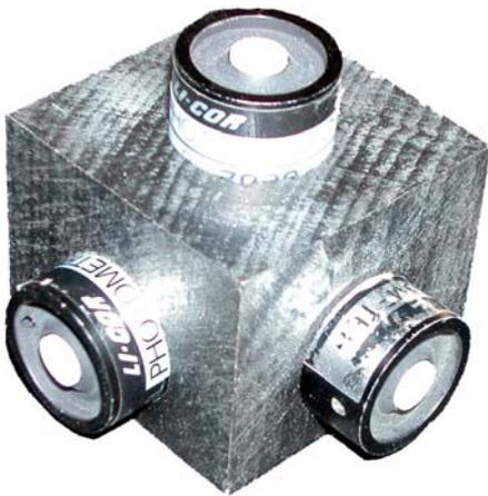
*Fig. 1.10. Illuminance sensors fixed on a black wooden cube*
