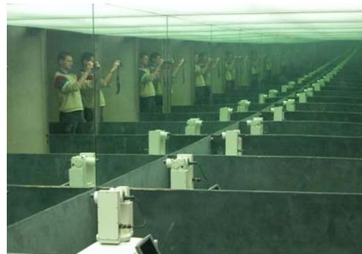
*Fig. 1.6. Picture of the sky scanner under artificial sky*
