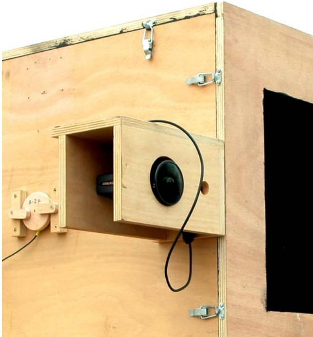
*Fig. 5.4. Digital camera with fish-eye lens for outdoor luminance measurements*
