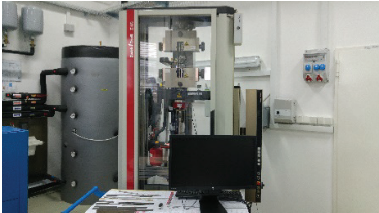
Figure 1: Universal Testing machine Zwick Roel, 100KN, testing of all kinds of materials
