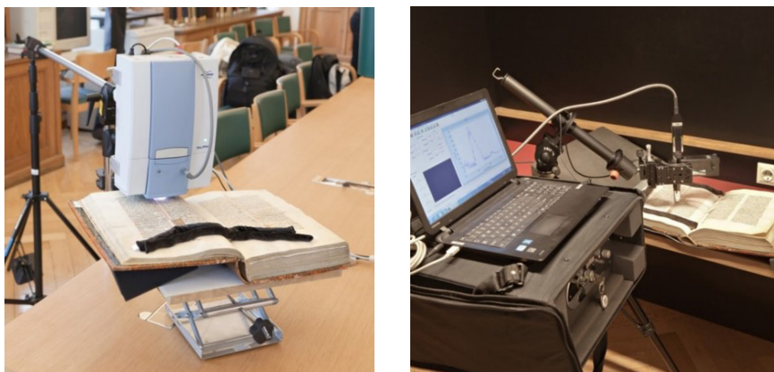
Fig. 6: The rFTIR-system Alpha (Bruker Optics, Ettlingen, Germany) (left) and the Raman spectrometer (Enwave Optronics, USA) at the Austrian National Library, Vienna (right).
