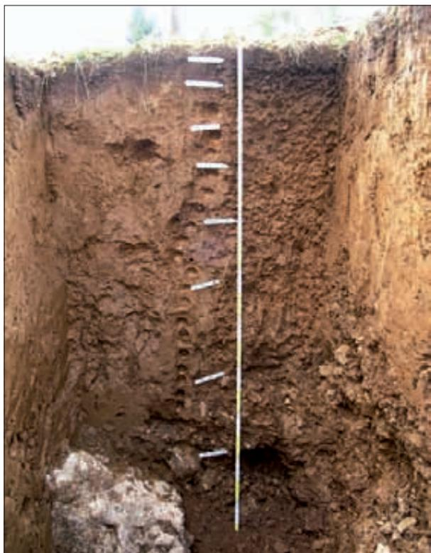
Fig. 7: The trench excavated in doline D29 showing the cavities of the sampling for the analysis.
