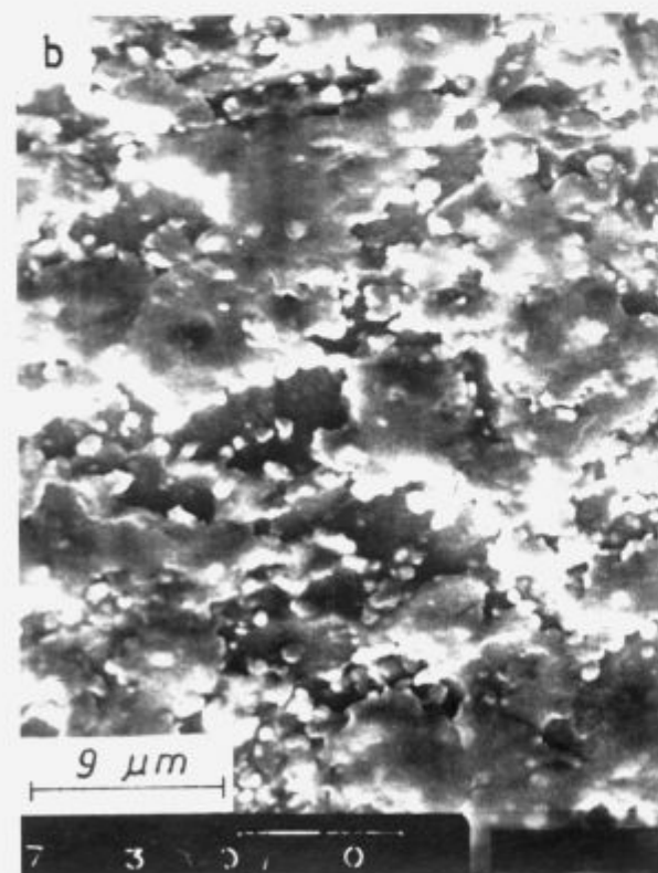
Figure 3: The microstructures tubings from low alloy Cr-Mo steel in as-rolled (a) and quenched and tempered state (b)
