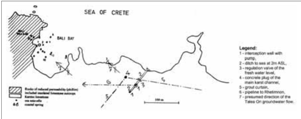
Fig. 14: Structures for the desalination of the Bali bay springs and estavelles (2008). Bali bay springs and estavelles (Economopoulos 1983).
