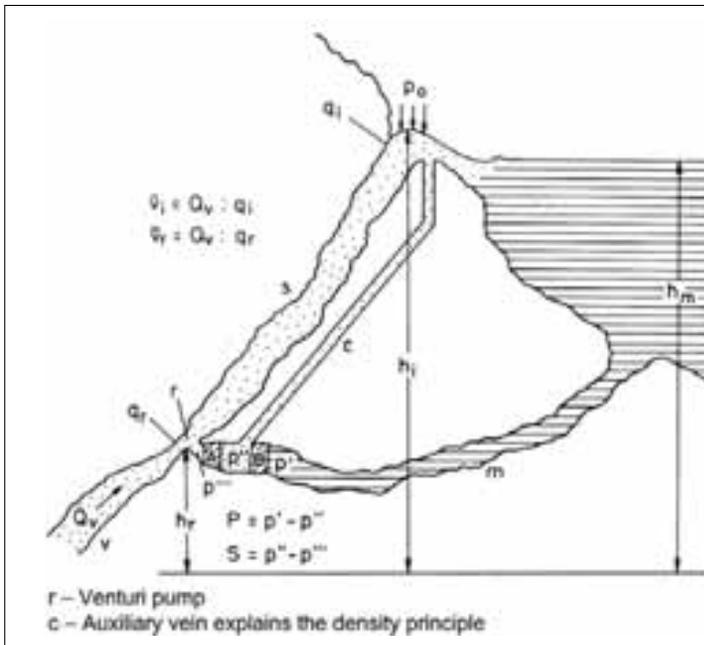
Fig. 4: Coastal spring of a conduit type (Kuščer 1950).
