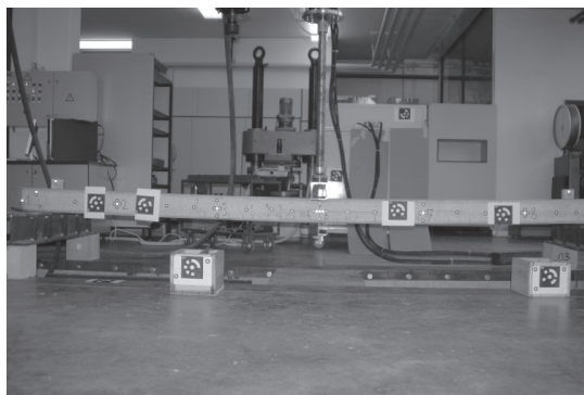
Fig. 3. Prefabricated prestressed concrete plate with measured marks
