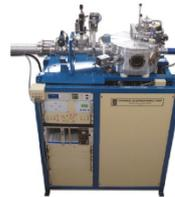
Analysis endstation that can include detector for RBS, Channeling, ERD, PIXE, PIGE, NRA, and IBIL. Offers monolayer depth resolution and sensitivity to  $10^{12}$  atoms/cm<sup>2</sup>. Optional microRBS and microPIXE systems are available.
