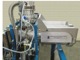
Single and multi-wafer implant chambers are available as well as custom chambers based on user specifications. Typical implantation range from  $10^{12}$  to  $10^{17}$  atoms/cm<sup>2</sup>
