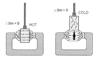
Fig. 1: Schematic illustration of the magnetocaloric effect
