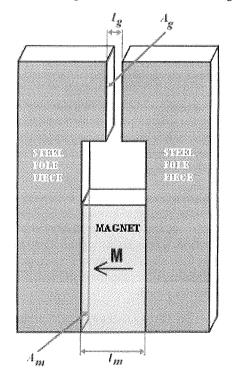
Fig. 2: Example of a simple magnetic circuit
