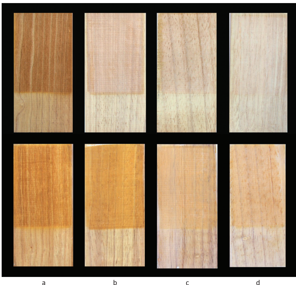
Figure 5. Colour changes after 1000 h of UV exposure of (a) uncoated, and coated with (b) 2 %, (c) 4 % and (d) 6 % \text{CeO}_2 (Top: without PU; Bottom: in PU coating).
