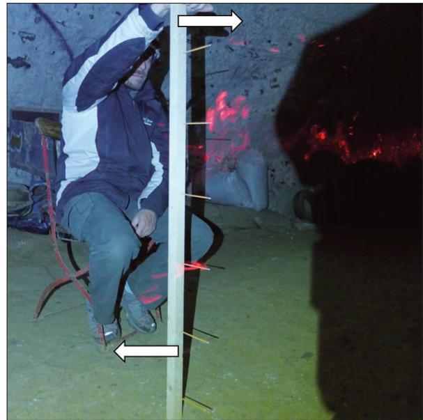
Fig. 3: In situ visualisation of airflow using a laser sheet. The smoke into the red plane of light is clearly visible. Arrows indicate the opposite directions of flows (Photo: L. Magne).
