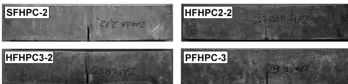
Figure 6: Notched FHPC samples after the test Slika 6: Vzorci FHPC z zarezo po preizkusu
