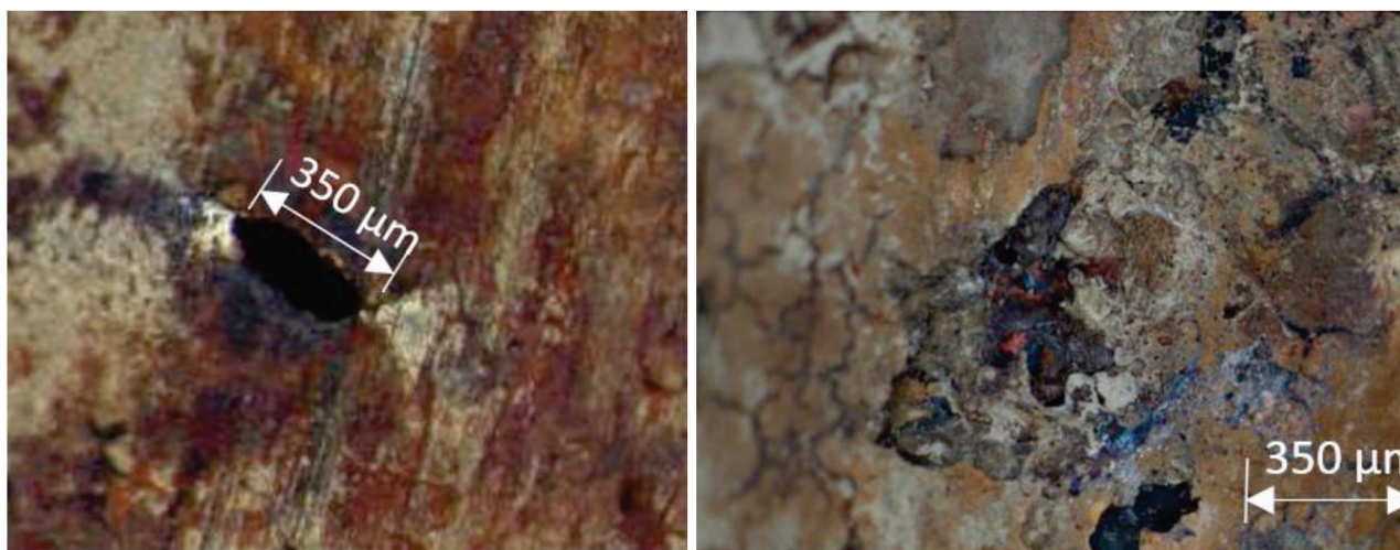
Figure 2: Microscopic images of the investigated rupture at: a) the steam side of the tube and b) the water side, magnification of 50×
