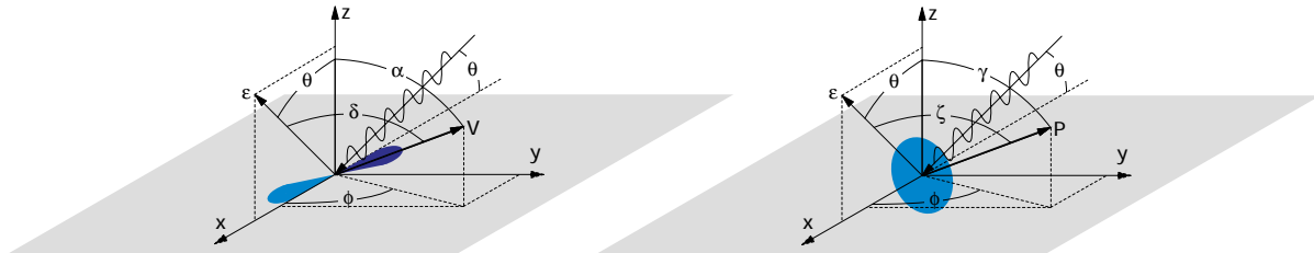
Figure 3.10: Coordinate system with the corresponding geometry of vector (left) and plane \sigma^* or \pi^* orbital on the surface.
