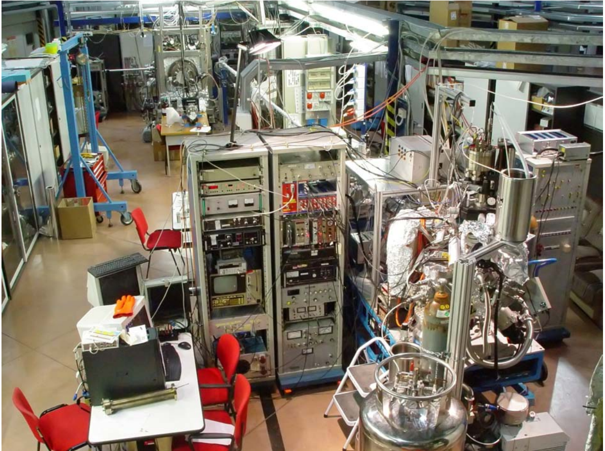
Figure 4.4: A photograph of the ALOISA/HASPES beamline (view towards the synchrotron beam source). The HASPEX experimental chamber can be seen in the front and the Aloisa experimental chamber in the back.
