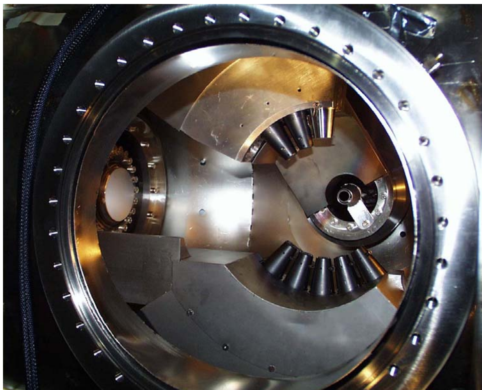
Figure 4.6: The photograph of the Aloisa main chamber. The SR beam impinges horizontally from the right hand side. The bimodal frame (top) and the axial frame (left/bottom) can be seen.
