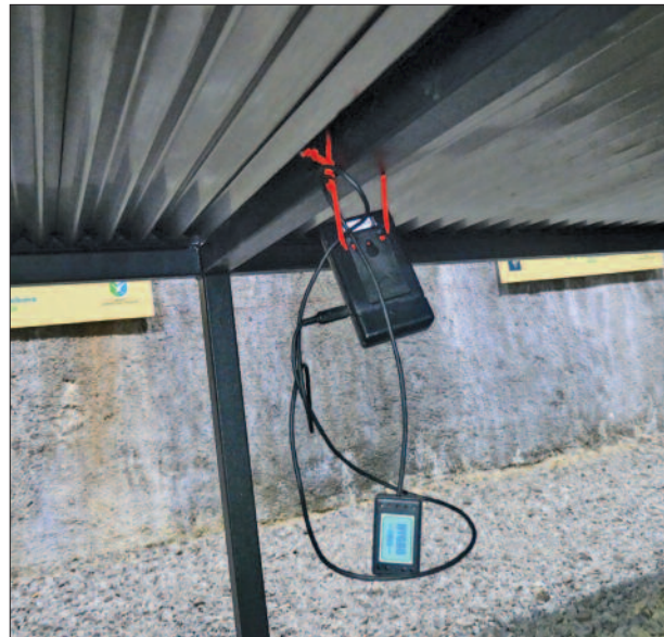
Slika 1. Senzor za spremljanje temperature in relativne zračne vlažnosti v bunkerju Goli vrh. Figure 1. Sensor for monitoring of the relative humidity of air and temperature in the underground fort Goli vrh.
