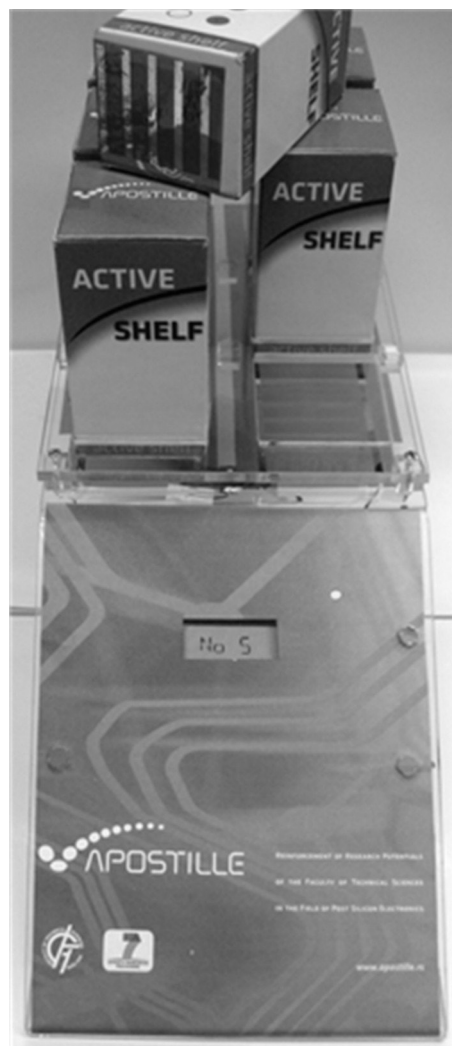
Figure 12: Developed platform of the counter of the number of products on the shelf.
