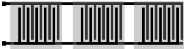
Figure 2: Ideal position of electrodes shown for tree IDCs.
