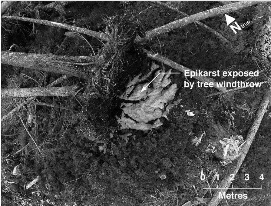
Fig. 4B: Low-altitude UAV image of the epikarst in the tree retention area exposed by the tree windthrow.
