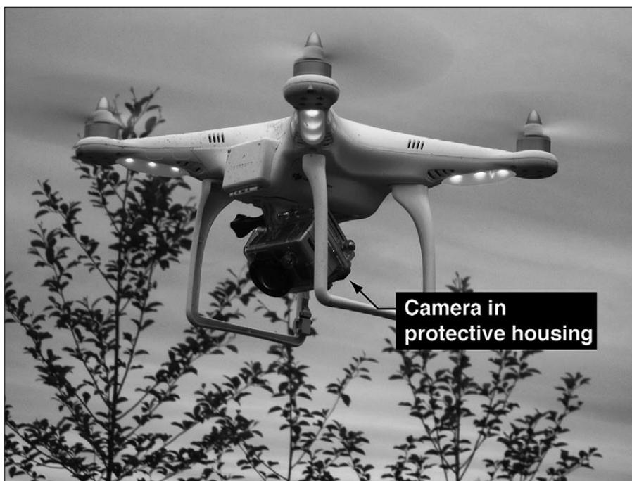
*Fig. 1: Mini multi-rotor UAVs equipped with compact high-resolution cameras are inexpensive and have the potential to increase data collection and monitoring capacity for karst researchers and managers (Photo: C.L. Ramsey).*
