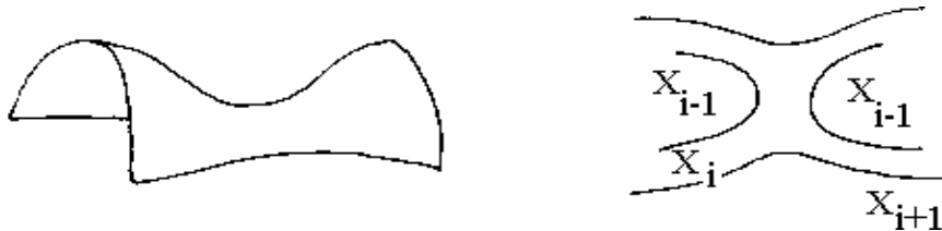
Fig. 2. Saddle configuration and corresponding thresholds.
