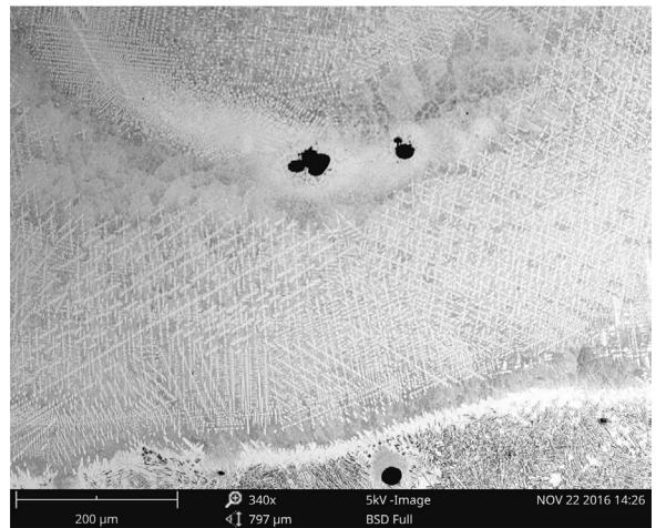
**Fig. 7.** Low magnification SEM image showing the non-uniformity in the microstructure on the cross-section of the SB no. C4
