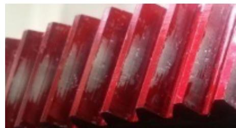
Fig. 12. Actual contact area of modified gear
