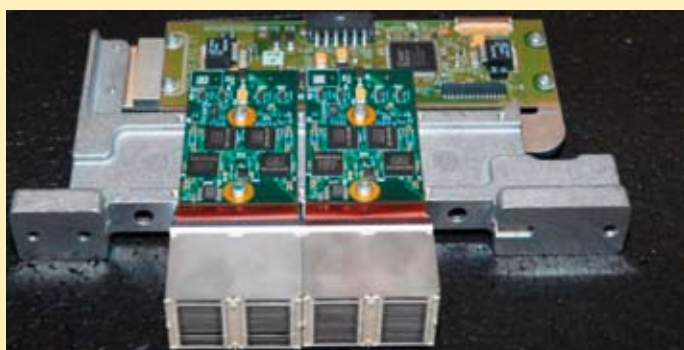
Figure 2: Prototype configuration of a second-generation detector module includes anti-scatter collimator, scintillator layer, photodiode array and a separate electronic board with ADCs
