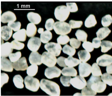
Fig. 2. Optical microscope image showing the rounded shapes of the sand grains.
