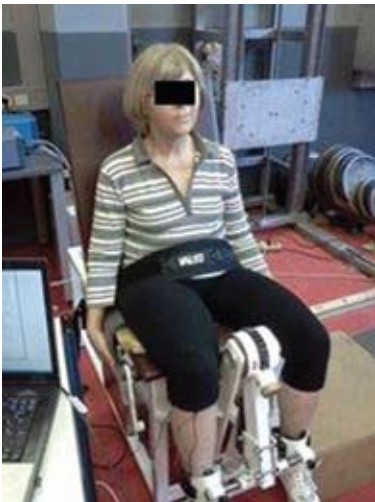
Figure 1: The isometric knee extension dynamometry
