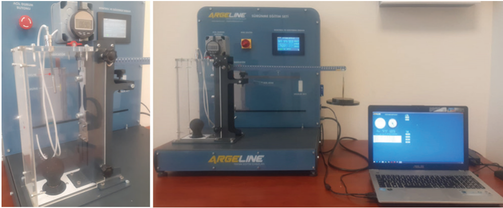
Fig. 2. General view of the creep test device and detailed view of the test region
