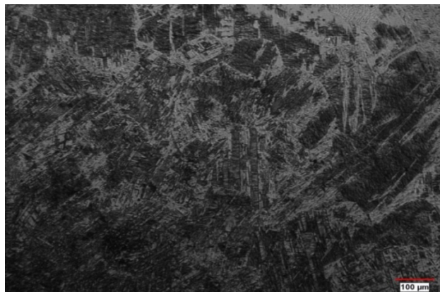
Fig. 10 Optical micrograph at 100x magnification of heat-treated manganese steel worn out- surface with evidence of high work hardenability after wear test
