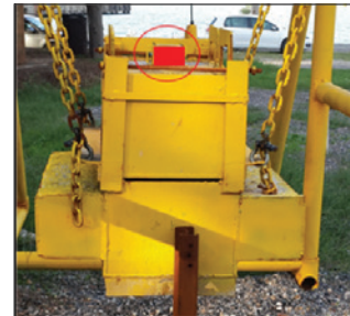
Figure 5. Pendulum test device used in dynamic impact tests with three dimensional accelerometer.
