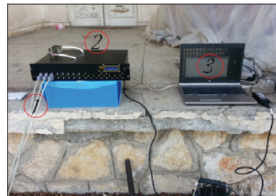
Figure 6. Data acquisition setup used during dynamic pendulum testing (1) data cable between accelerometer and data collector box, (2) 8-channel data collector, (3) recording data in a computer.
