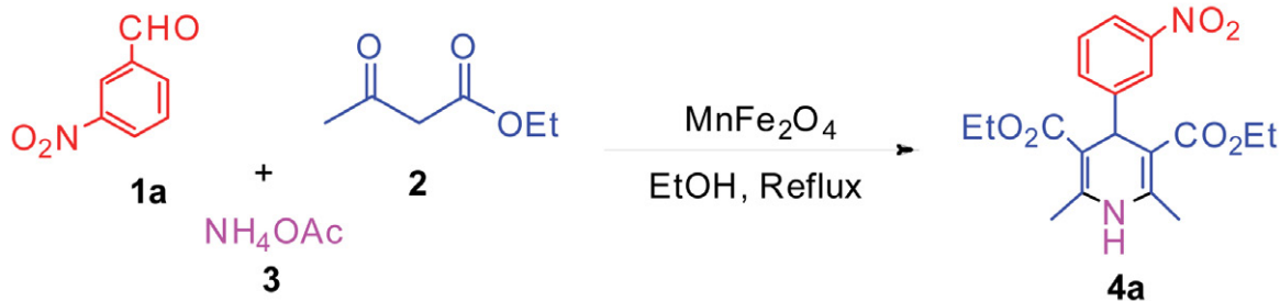
Scheme 1. Model reaction for the synthesis of diethyl-1,4-dihydro-2,6-dimethyl-4-(3-nitrophenyl)pyridine-3,5-dicarboxylate.
