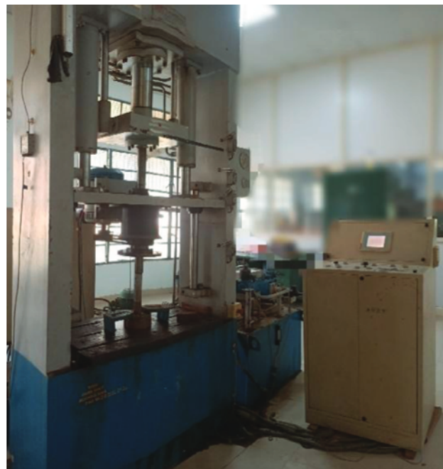
Figure 3: PLC-operated 100-ton hydraulic press
