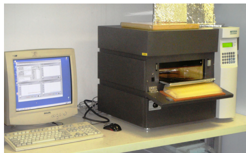
Fig. 4. Laboratory measurement of thermal conductivity
