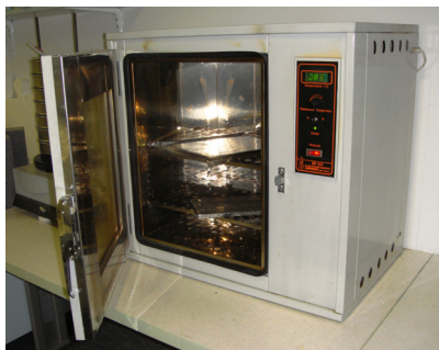
Fig. 3. Oven for accelerated ageing temperature stress
