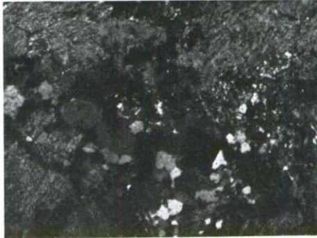
Fig. 3. Amphibolite (grains of hornblende in groundmass of salic minerals)  $\times 35$ . Gayo Camp. Determination A. Hinterlechner
