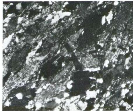
Chlorite-talc-tremolite schist forms the next zone of Ula Ulo and farther south in the Ujima area. The rock is composed of an association of talc, chlorite, and tremolite. The size of mineral grains is less than 0,1 mm. Magnetite is accessory only; its crystals range in size from 0,03 to 20 mm. A parallel structure of bands of chlorite and talc could be observed. The rock is a product of the regional metamorphism of the sediments.
