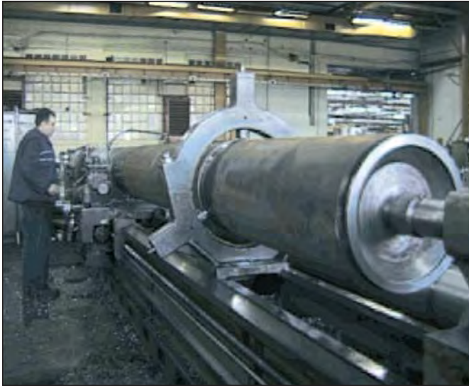
Figure 1. Honing machine "WDF"
