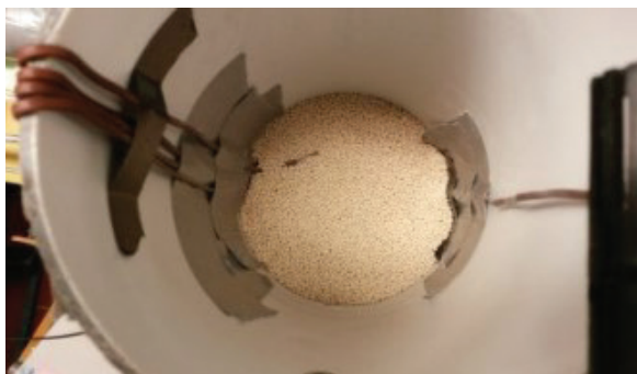
Fig. 3. Adsorber with bulk of zeolite 13X
