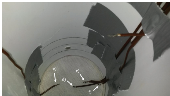
Fig. 6. Measurement points of the temperatures that were measured at the bottom of zeolite bulk
