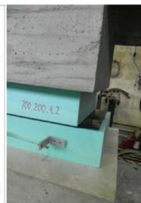
Figure 7: Scheme of a TI foundation set with a HI sheet between two XPS boards, and the building's possible seismic response (sliding).
