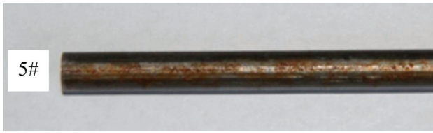
Figure 7: Surface of AWJ specimen No. 5 after 24 h of AASS
