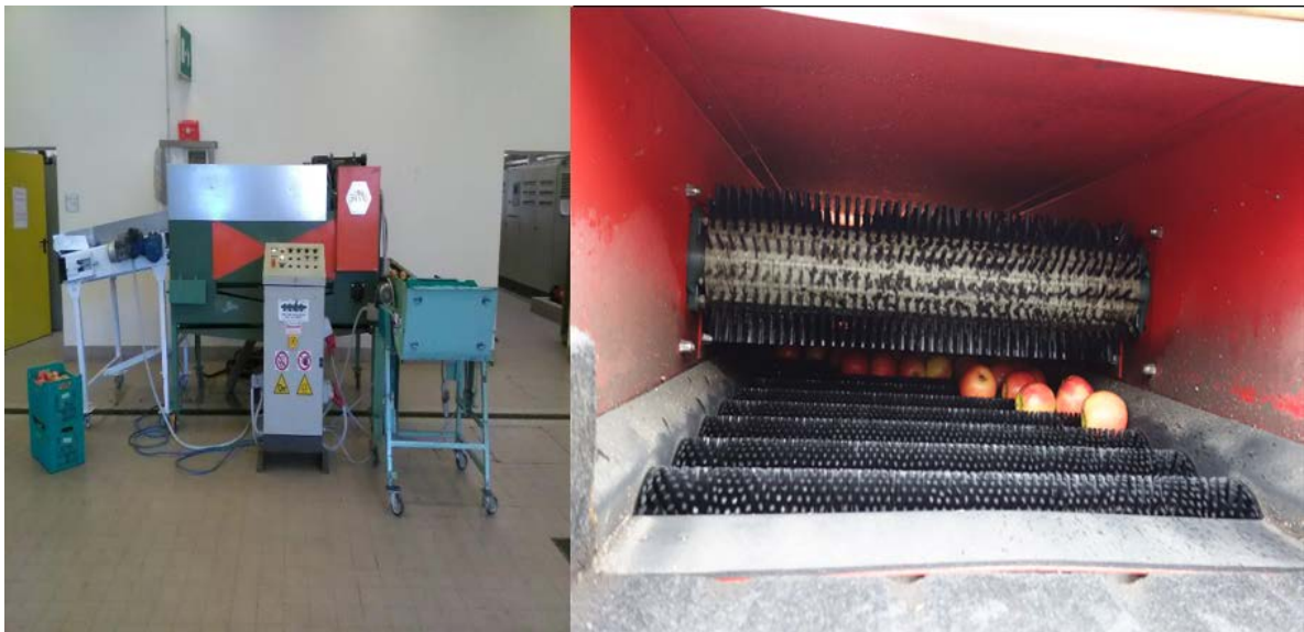
Figure 2: prototype of apple brush from the Valentino company (Italy) Quelle: Valentino company
