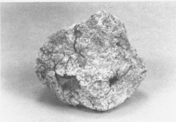
Slika 1: Zrno žlindre razpokano zaradi povečanja volumna zm dikalcijevega silikata pri prehodu iz \beta v \gamma obliko Figure 1: Cracked grain of slag caused by volume increase of dicalcium silicate grains between transformation from \beta into \gamma modification
