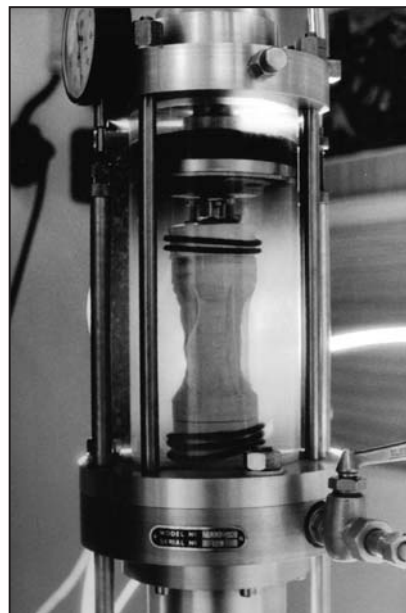
Figure 15. Photo of tested Most clay with visible two necks.
