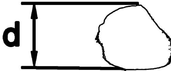
Figure 2: Cross-sectional area of potato stalk with marked dimension d
