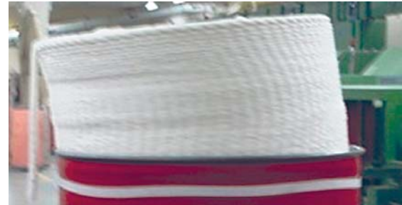
Figure 4: Can-spring buckling on sliver storage in older can
