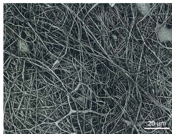
Figure 2: CLSM image of PAN/gelatine nanofibrous mat with 10% gelatine after electrospinning; scale bar indicates 20 \mu m
