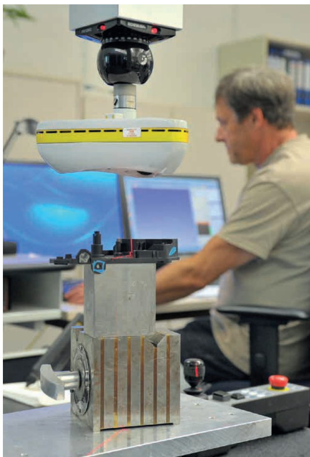
» Operater programira pot skeniranja s programsko opremo Focus.
