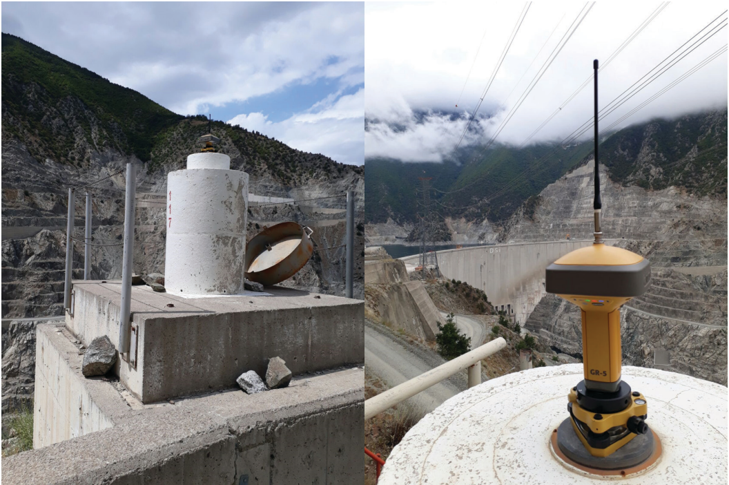
Figure 3: GNSS receivers on reference points 117 (left) and 104 (right).
