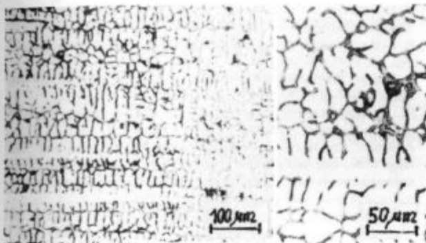
Slika 5: Mikrostruktura navara z enojno elektrodo "EPP 2" pod praškom "U-Mo 6" - feritna z maloogljčnim martenzitom Figure 5: Microstructure of a surfacing made by submerged arc surfacing with single electrode "EPP 2" and flux "U-Mo 6" - ferrite with low-carbon martensite
