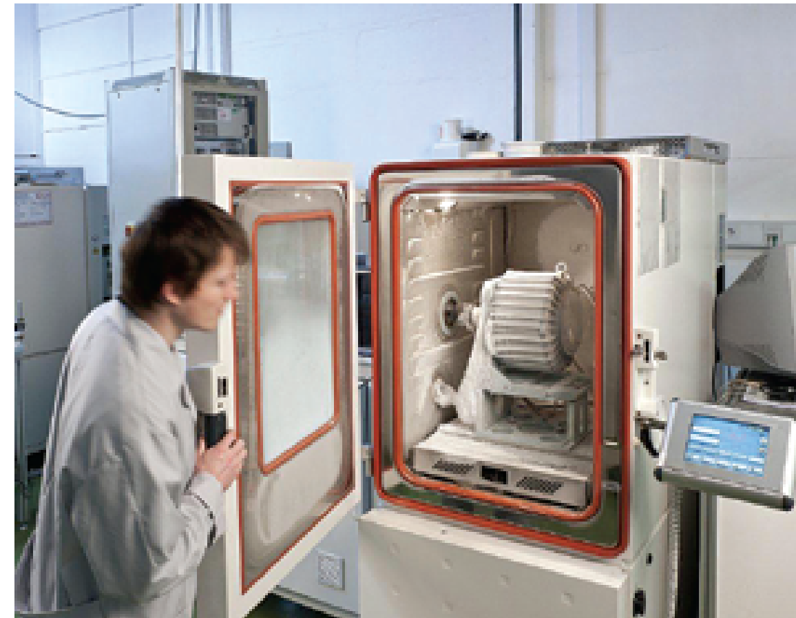
Motor at -40°C in the temperature shock test chamber
