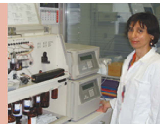
Figure 3: the Procise 492A protein sequencing system (Applied Biosystems) has been completely renewed to meet the needs of contemporary protein primary structure analysis.
