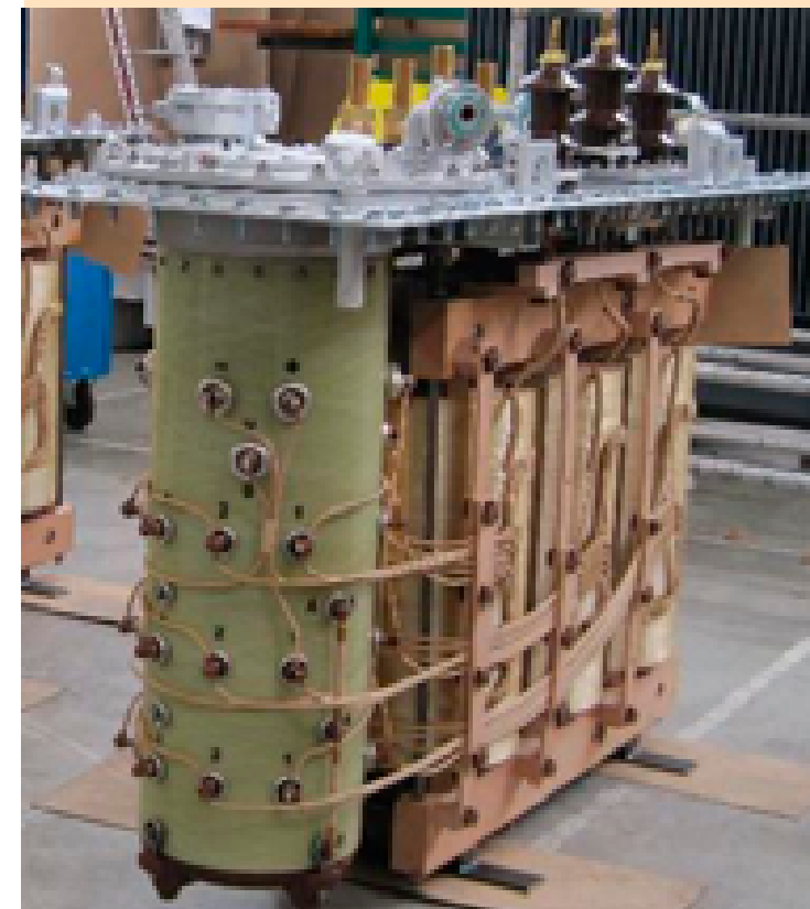
Active part of a distribution transformer incl. regulation of voltage under load.
