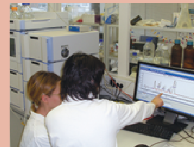
Figure 4: the Flexar FX-15 UHPLC system (Perkin Elmer) is a liquid chromatography system used to prepare peptide samples for automated Edman sequencing.
