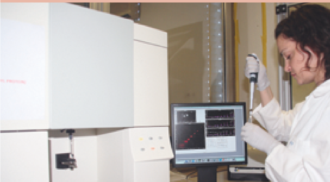
Figure 1: the flow cytometer (BD FACSCalibur) system is a renowned bench-top flow cytometer with a modular design, which has a proven record of performance, sensitivity and flexibility, and has been a valued tool in research and clinical laboratories worldwide for a number of years.
