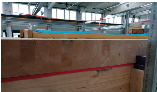
Fig.1. Test suite at TU Vienna with tested floor and flanking path decoupling with flexible interlayers
