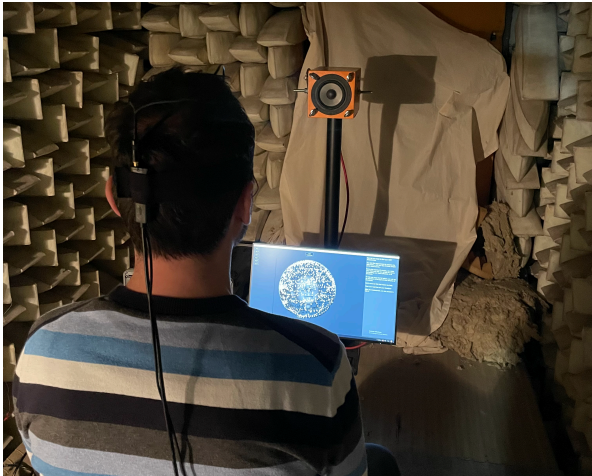
Fig.1. HRTF measurement in the anechoic chamber
