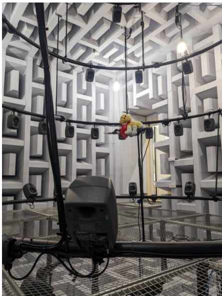
Fig.6. Listening test in the anechoic chamber at InnoRenewCoE
