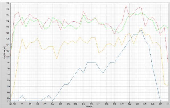
Fig.10. Open window measurement: no filtering (red), band-pass filtering 1 Hz to 20 Hz (green), band-pass filtering 20 Hz to 40 Hz (orange), and car speed in km/h (blue). LabVIEW software.
