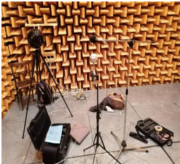
Fig.3. Comparison of the eigennoise of Eigenmike em32 Ambisonics microphone to a Norsonic 1225/1209
