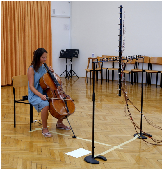
Fig. 1. The typical recording configuration for violoncello measurements. A microphone array of 33 microphones designed and built for this purpose was used. The positioning of the musician and the microphones was maintained between recordings.
