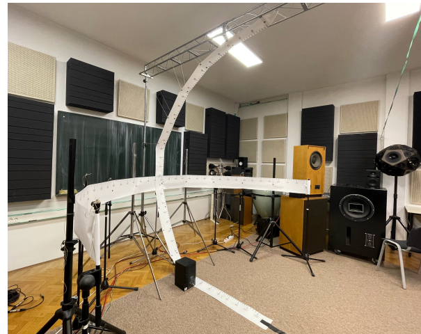
Fig.2. Horizontal and vertical paper tapes used for determining the azimuth and the elevation of the sound source
