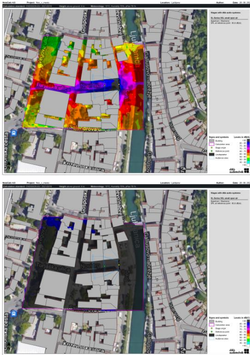
Fig 4.: dBA and dBC maps using spectrum of electronic music [7].
