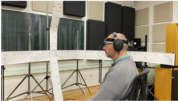
Fig.3. A participant with head-mounted binaural system elements on a rotating chair, tracking the virtual sound stimulus
