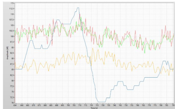
Fig.8. Closed window measurement: no filtering (red), band-pass filtering 1 Hz to 20 Hz (green), band-pass filtering 20 Hz to 40 Hz (orange), and car speed in km/h (blue). LabVIEW software.
