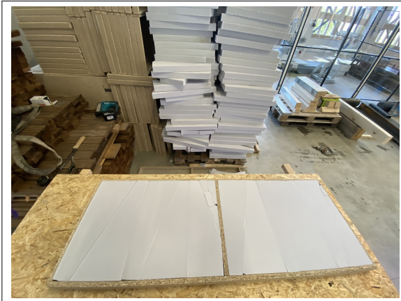
Fig. 1. Monolithic type of a sound absorber
