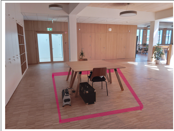
Fig. 3. Position of the tapping machine and walking path (pink) on the third floor of the InnoRenew CoE
