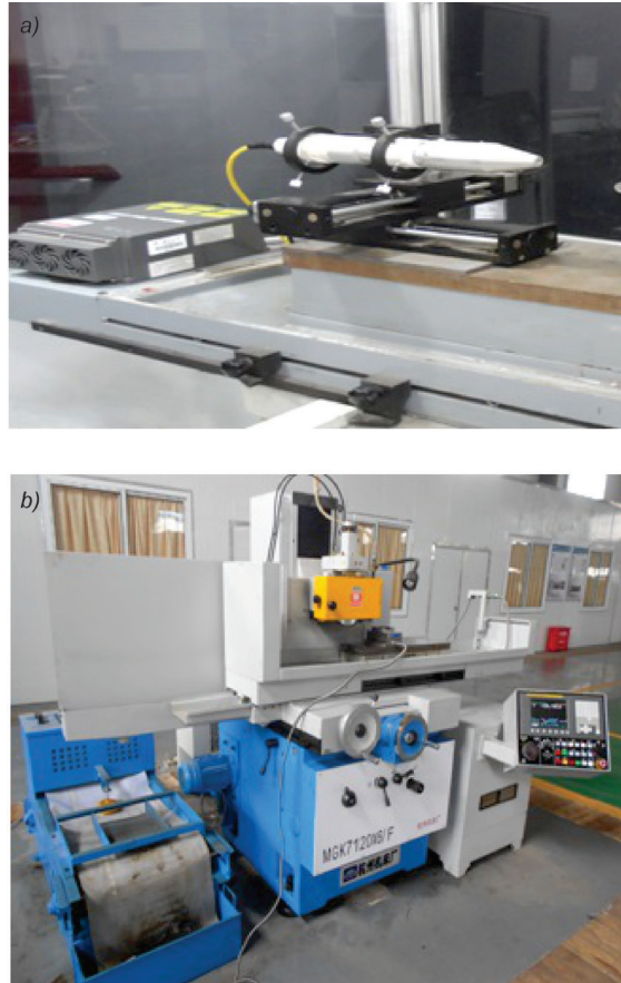
Fig. 4. a) The apparatus used for laser induced deterioration grinding; b) a detail
