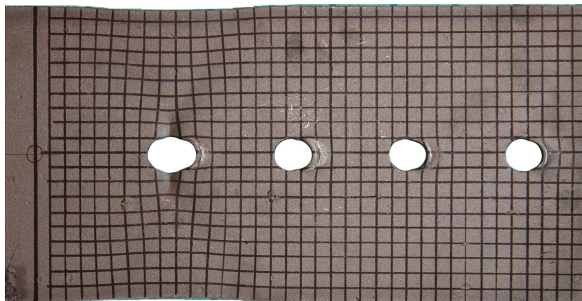
Fig. 29: Net cross-section failure of specimen L20
